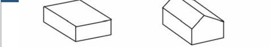
**Fig. 3:** Different geometry LODs. Left: Cube model. Centre: Main roof. Right: Detailed roof.
