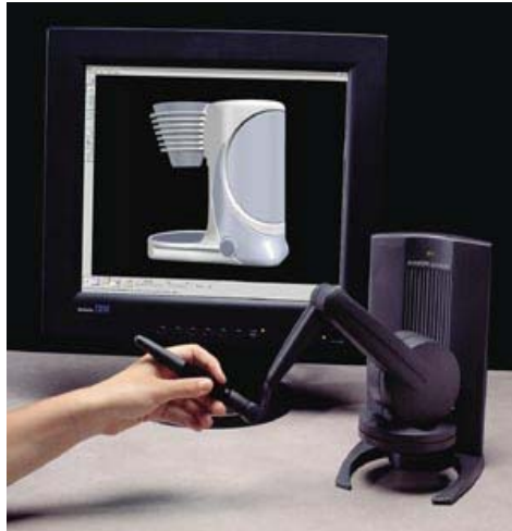
Figure 1. PHANTOM™ Desktop from SensAble Technologies is a popular linkage-based haptic device. The position and orientation of the pen are tracked through encoders in the robotic arm. Three degrees of force, in the x , y and z , direction are achieved through motors that apply torques at each joint in the robotic arm.
