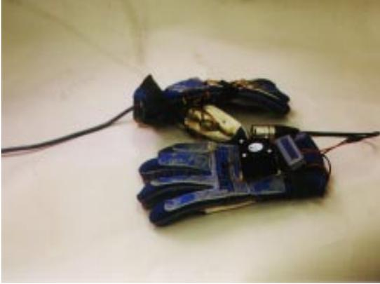
**Figure 73. Tactile Feedback Glove
