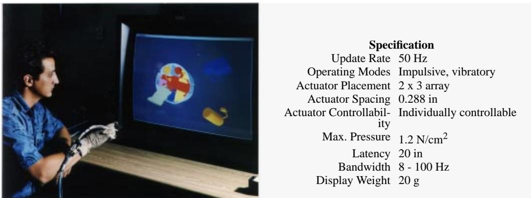
Figure 71. Tactile Display (Sandia National Laboratories)
